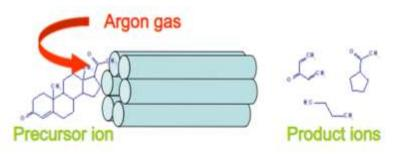
In the collision cell, the TRANSLATIONAL ENERGY of the ions is converted to INTERNAL ENERGY.
